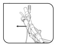
Position the white front reflector to the right of the handlebar stem so that it points directly forwards and is within 5 degrees of the vertical. Attach the bell in the same manner to the left of the handlebar stem.
