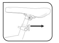
Position the red rear reflector on the seat post so that it points directly backwards and is within 5 degrees of the vertical.
