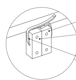
1 Step: Attach one supplied timber block to the back of the unit. Use 2 x G screws.
