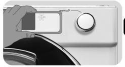
If you do not know the position of your NFC antenna, slightly move the smartphone in a circular motion over the ONE Fi EXTRA logo until the App confirms the connection. In order for the data transfer to be successful, it is essential TO KEEP THE SMARTPHONE ON THE DASHBOARD DURING THESE THE FEW SECONDS OF PROCEDURE; a message on the device will inform about the correct outcome of the operation and advise you when it is possible to move the smartphone away.
