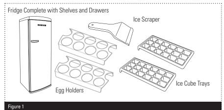
This illustration is only for information about parts of the appliance. Parts may vary according to the appliance model
