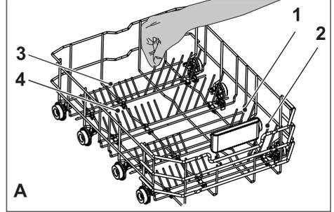
To bring the collapsible tines into horizontal position, grab the tines from mid position and push them in the directions of arrows (B). To bring the tines back to vertical position, just lift them up. Collapsible tines will click into the latch again.
