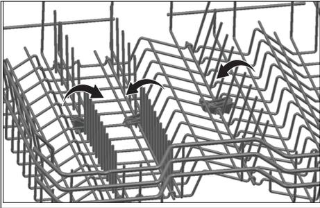
**i** Bringing the wires to the horizontal position by holding them from the tips may cause them to bend. Therefore, hold the wires from their stems while bringing them to the horizontal or vertical positions.
