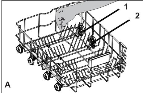
To bring the collapsible tines into horizontal position, grab the tines from mid position and push them in the directions of arrows (B). To bring the tines back to vertical position, just lift them up. Collapsible tines will click into the latch again.
