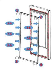
After the replacement check if there any nonfitting point on the gasket. Also check if there any opening at the gasket while the door is closed. If so that might cause condensation/icing or insufficient cooling/freezing. To prevent this soften the form of the gasket with the help of a hair dryer or hot water and make sure that all points are closing perfectly.
