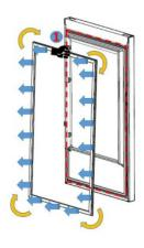
Check the replacement gasket from starting with upper right corner, press on the gasket until it fits to its place. Place the other sides of the gasket with the help of your thumb
