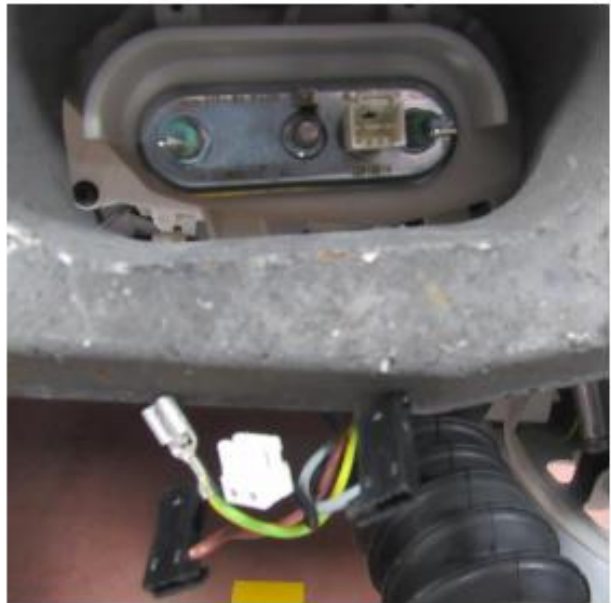
Remove the heater sockets
