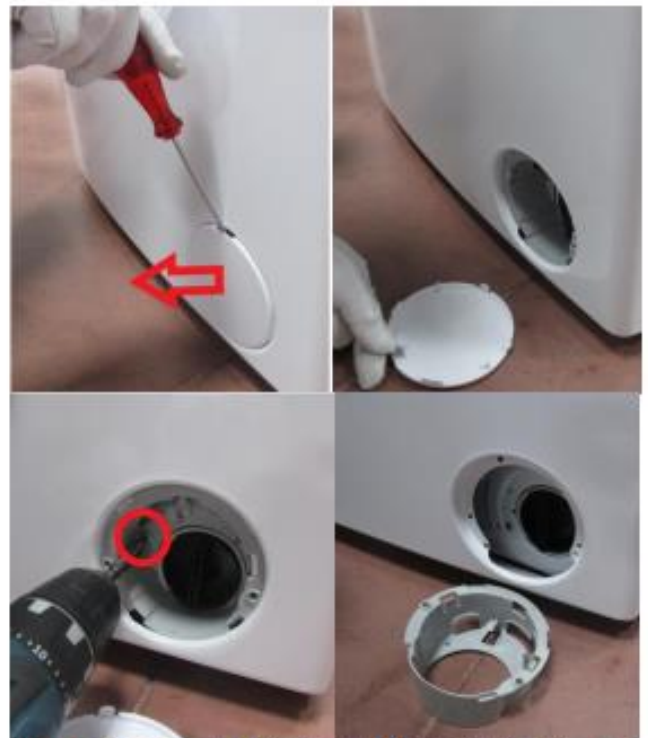
Remove the screw and plastic part located under the pump cover
