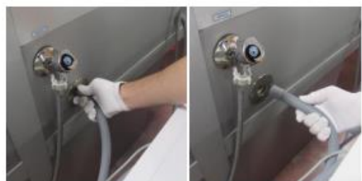
Disconnect the drain hose
