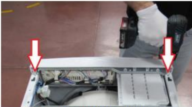
Remove two screws fixing control panel.
