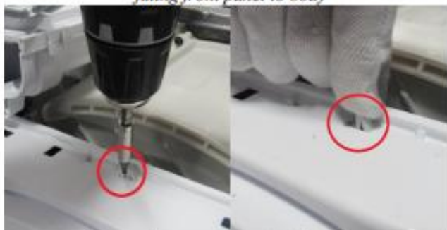
Remove the screw fixing twinjet elbow.
