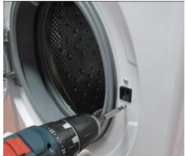
Remove the screws fixing the door lock.
