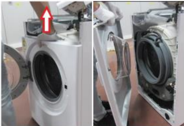
Pull up and remove the front panel.
