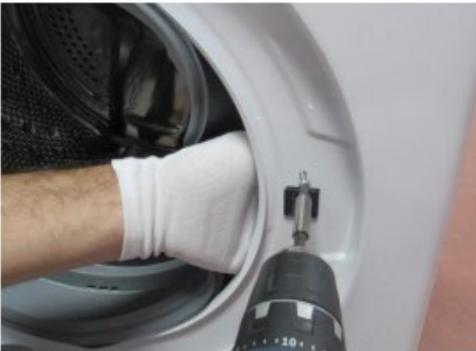
Tighten the door lock screw
