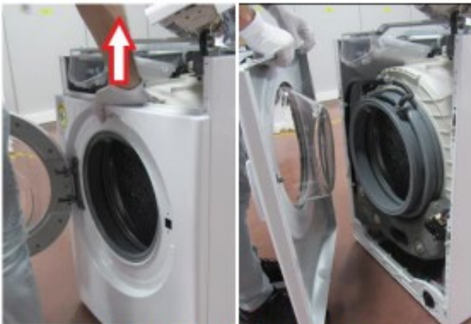
Pull up and remove the front panel.
