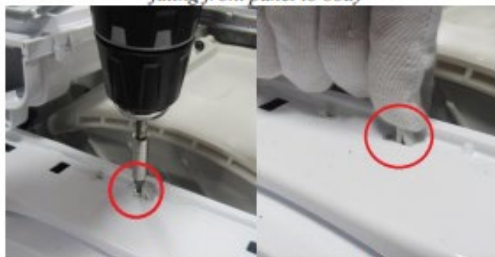
Remove the screw fixing twinjet elbow.
