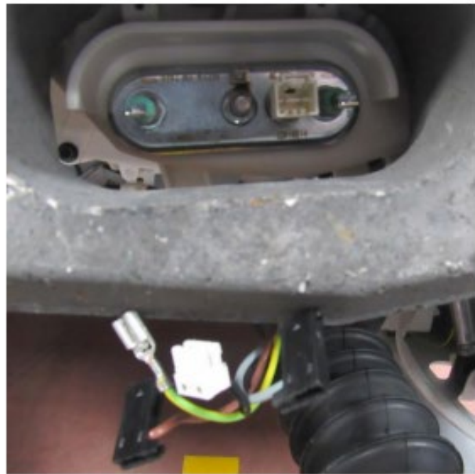
Remove the heater sockets
