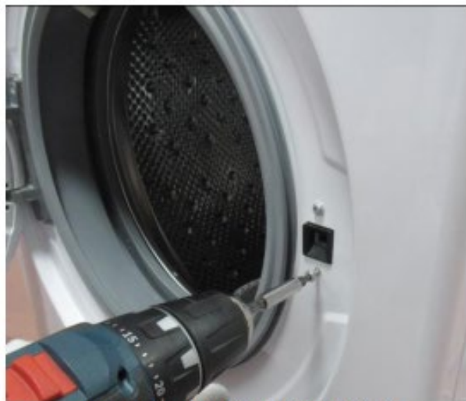
Remove the screws fixing the door lock.
