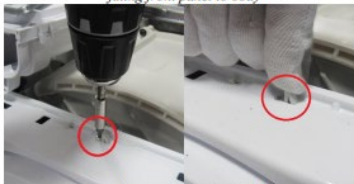
Remove the screw fixing twinjet elbow.
