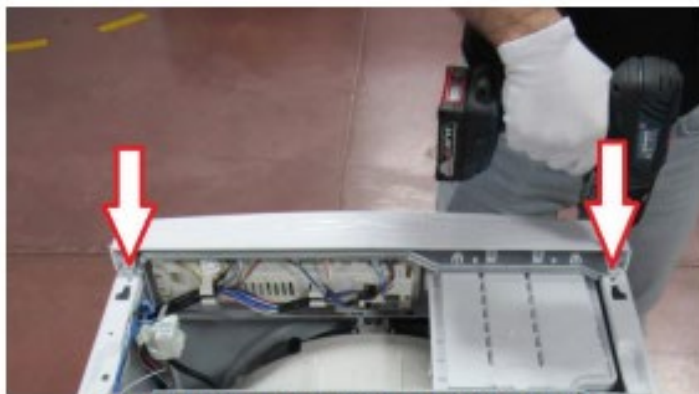
Remove two screws fixing control panel.
