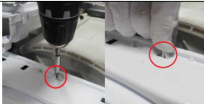
2.5. Remove the screw fixing twinjet elbow.
