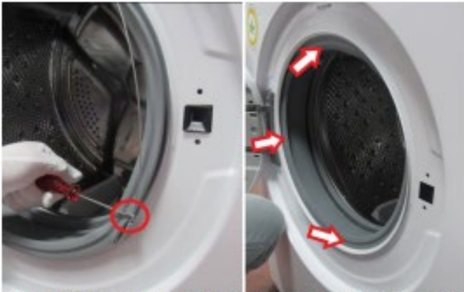
Remove the wire by using small screwdriver and push the seal to the inside
