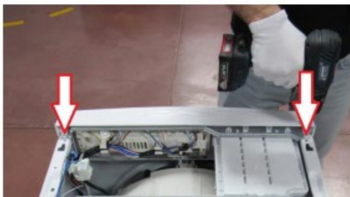
Remove two screws fixing control panel.
