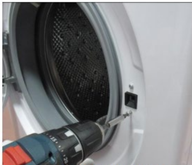
Remove the screws fixing the door lock.
