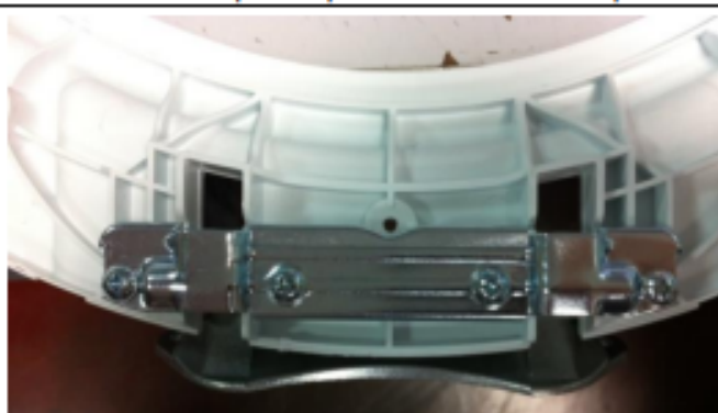
2.8. Remove the hinge sheet by screwdriver
