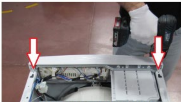
Remove two screws fixing control panel.
