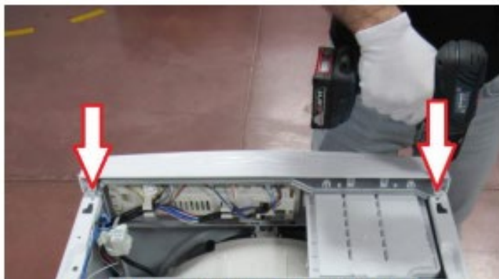
Remove two screws fixing control panel.
