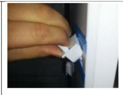
After the switch is placed, complete the assembly by pushing.
