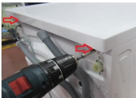
Remove two screws that fix the top-plate at the back.
