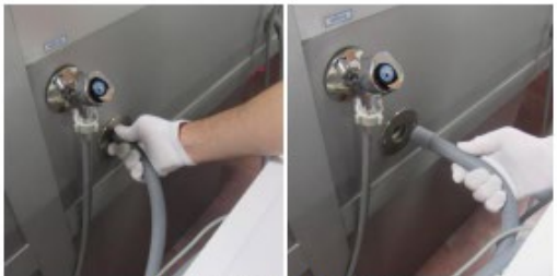
Disconnect the drain hose
