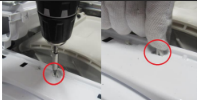
2.5. Remove the screw fixing twinjet elbow.
