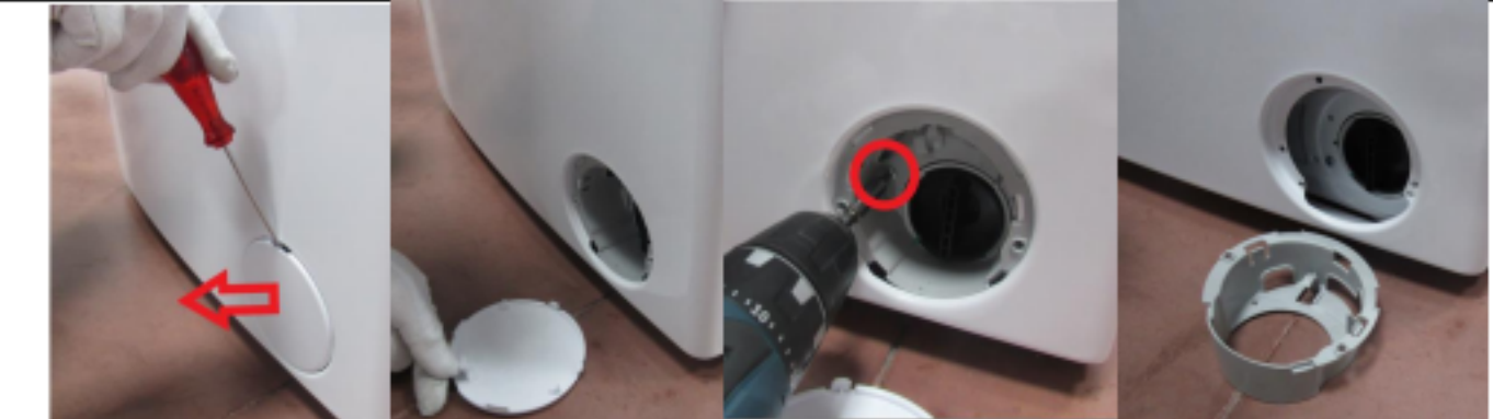
2.7. Remove the screw and plastic part located under the pump cover
