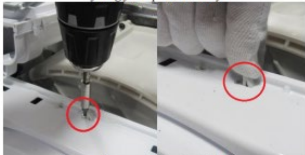
Remove the screw fixing twinjet elbow.
