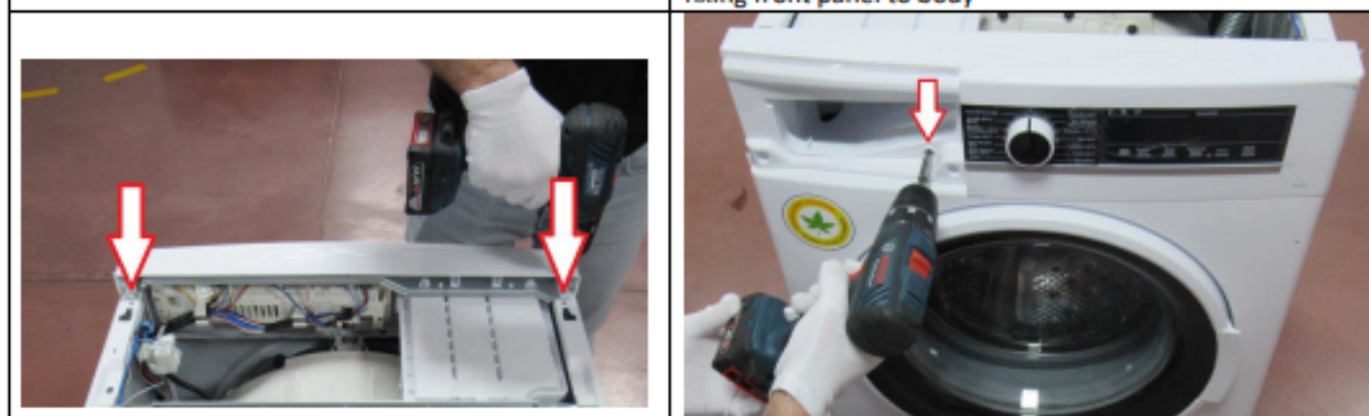
3.9. Tighten the screw on support bracket and two screws fixing front panel to body
