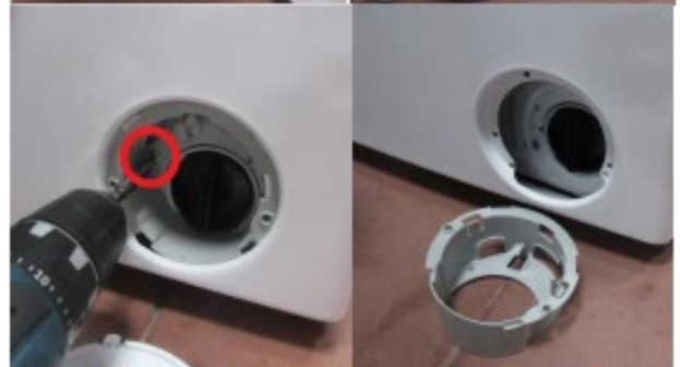
Remove the screw and plastic part located under the pump cover
