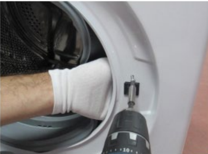
Tighten the door lock screw
