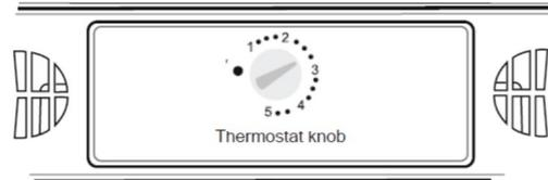
The freezer thermostat automatically regulates the temperature inside the compartments. Cooler temperatures can be obtained by rotating the knob to a higher number (1 to 5). The “•” position closes the thermostat so no cooling will take place.
