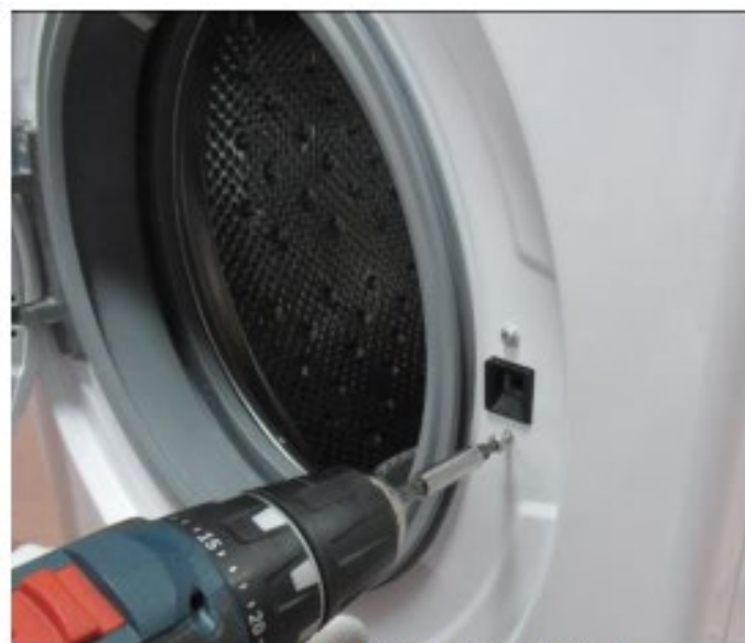
Remove the screws fixing the door lock.
