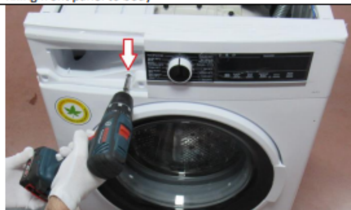
3.9. Tighten the screw on support bracket and two screws fixing front panel to body
