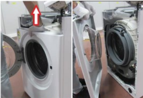
Pull up and remove the front panel.
