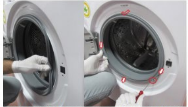
Pull the tub bellow seal to the outside and assemble the wire by using small screwdriver
