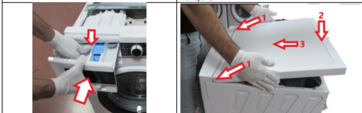
3.12. While pressing siphon cover keep pushing
