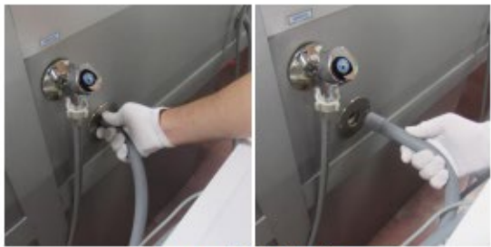
Disconnect the drain hose
