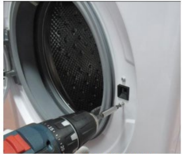
Remove the screws fixing the door lock.
