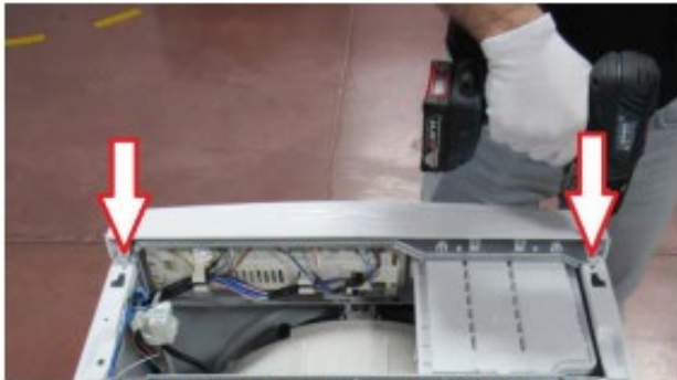
Remove two screws fixing control panel.
