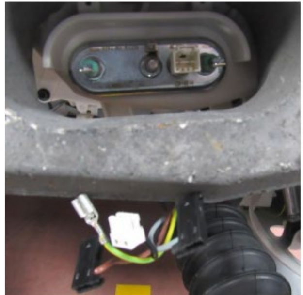
Remove the heater sockets
