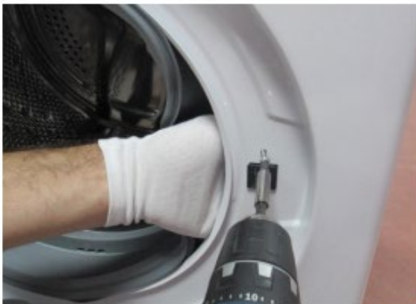
Tighten the door lock screw
