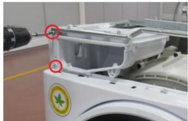
Remove the screw on support bracket and two screws fixing front panel to body
