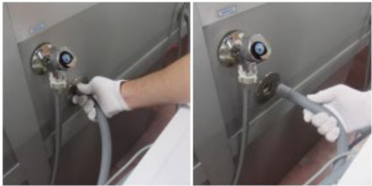
Disconnect the drain hose
