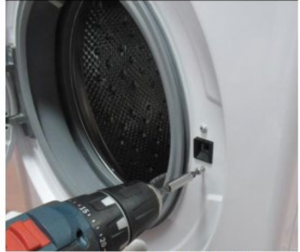
Remove the screws fixing the door lock.
