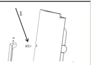
2) Install the door handle onto the bolt, tighten the screw in the handle side hole with the Allen wrench in the plastic bag, install the screw cover, and complete the installation.
