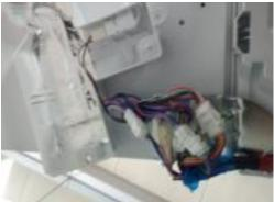
2) Disconnect the connectors, then use cross screwdriver or socket spanner to remove the 2pcs M5 screws and 1 pc grounding screw by anticlockwise, then remove the upper hinge.
