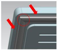
2)Take efforts until door seal totally detaches from door inner liner groove, remove the door seal
