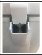
2) Hold the side of upper hinge cover with both hands, align the opening with the side wall of the hinge, and push down until the hinge cover protrusion completely falls into the hinge hole. Then the upper and lower hinge covers are all in place.
