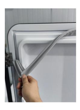
Step 2 Install a new gasket, starting from the fridge one corner.
