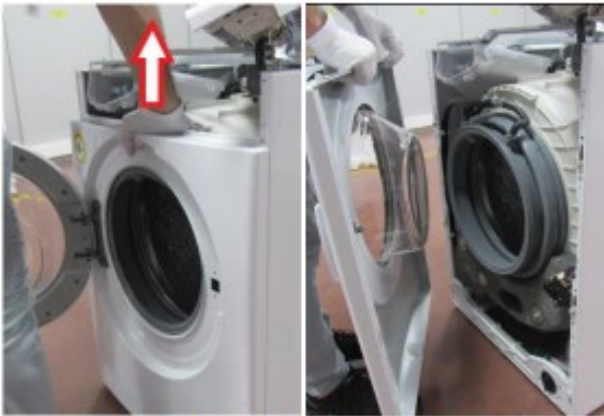
Pull up and remove the front panel.
