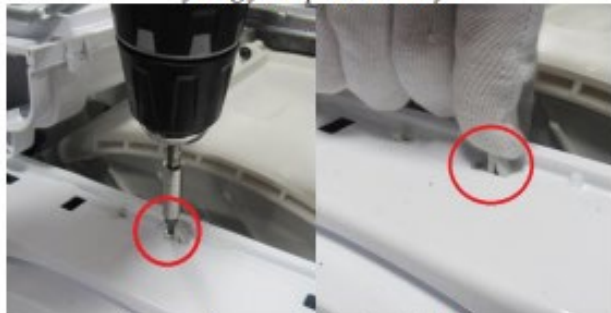
Remove the screw fixing twinjet elbow.
