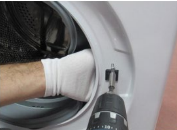
Tighten the door lock screw
