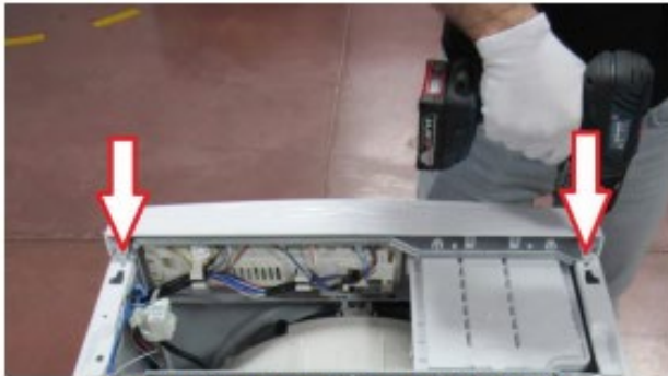
Remove two screws fixing control panel.
