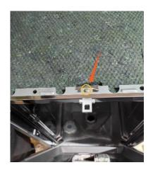
2. Remove the lock latch **Tool:** D. Phillips screwdriver (H6 or ∮ 6)
