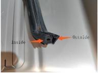
2.1 Install sealing strip in the direction shown;
