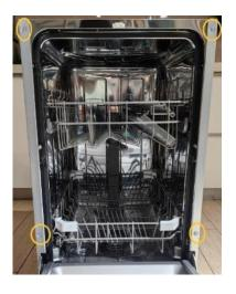
2. Remove screws from the side panels **Note:** If only one side of the hinge needs to be replaced, only the required side panel needs to be removed.
