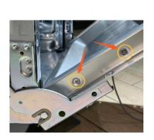
Use pliers to hold the door pull rope and remove it from the buckle of the hinge.
