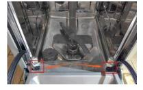
2.3 according to the figure, Install the sealing rings on both sides of the bottom first.
