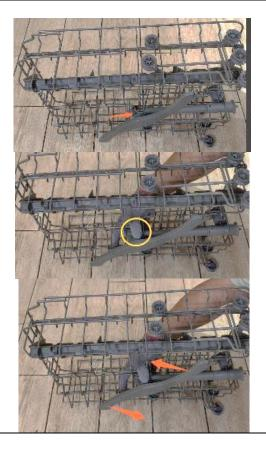
1. Replace the upper spray arm 1.1 Remove the upper bowl basket and pinch the position shown.
