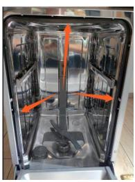
2.5 Press the seal rings around as shown. If not tightly pressed, there may be abnormal closing or water leakage.
