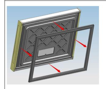
Take efforts until door gasket totally detaches from door liner groove, remove the door gasket.
