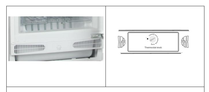
The freezer thermostat automatically regulates the temperature inside the compartments. Cooler temperatures can be obtained by rotating the knob to a higher number (1 to 5). The "•" position closes the thermostat so no cooling will take place.
