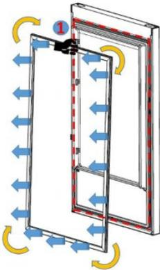
Check the replacement gasket from starting with upper right corner, press on the gasket until it fits to its place. Place the other sides of the gasket with the help of your thumb
