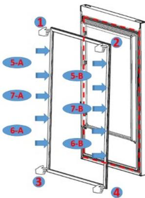
After the replacement check if there any nonfitting point on the gasket. Also check if there any opening at the gasket while the door is closed. If so that might cause condensation/icing or insufficient cooling/freezing. To prevent this soften the form of the gasket with the help of a hair dryer or hot water and make sure that all points are closing perfectly.
