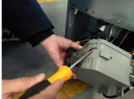
2)Disconnect all the wiring connectors.
