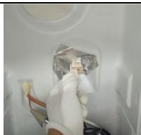
7) After the removal of upper air duct in freezing chamber. Catch hold of cover plate of freezing lower air duct shown in the picture, pull it out along the arrow direction and take it out.
