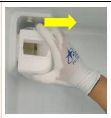
4) Remove connecting terminals of ventilation door and take out refrigerating air duct foam.
