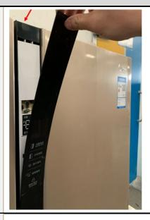
2) Use the tool to lift the display control assembly from the bottom.
