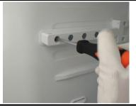
2) Remove aluminum foil on screw hole caps, then use knife to take off the screw hole caps.
