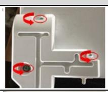
2) Press the snap joint in the circle and push it outward along the arrow direction. Complete the disassembly of door light switch.
