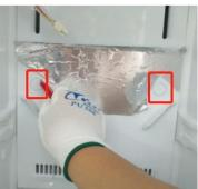
3) Remove the 2 fitting screws of upper front cover of freezer air duct.
