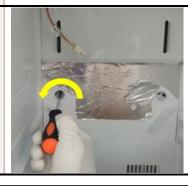
4) Hold the front cover and pull outwards with big force until it is separated from the liner.
