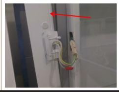
3) pull out the whole rollover beam to seperature the lower part from the door;
