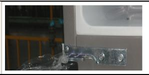
2) Then lift the freezer door up and away from the bottom hinge axis, then carry the door to a suitable place. Save the screws to reuse.
