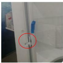
4) Unplug the wire terminal, remove the rollover beam, reverse the operation to complete the installation.
