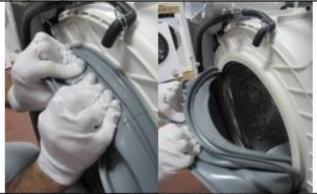
3.15 Hold the gasket bellows and the gasket body pull out in and out at the same time.
