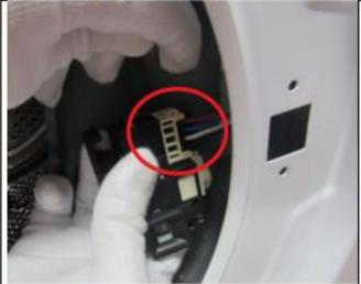
Unplug the connector and remove the door lock.
