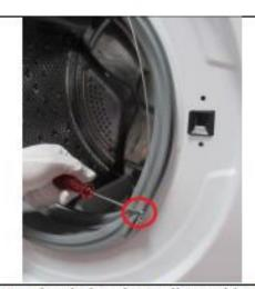
3.2. Remove the wire by using small screwdriver
