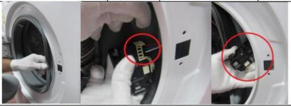
3.3. Remove the right side of the tub bellows seal and reach to door lock
