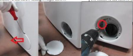
3.9 Remove the screw and plastic part located under the pump cover
