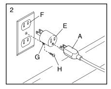
The lug (G) or wire extending from the adapter must be connected with a metal screw (H) to a permanent ground such as a properly grounded outlet box cover. Some 2-pole receptacle outlet box covers are not grounded. Before using an adapter, contact a qualified electrician to determine whether the outlet box cover is grounded. The temporary adapter should be used only until a properly grounded outlet can be installed by a qualified electrician.
