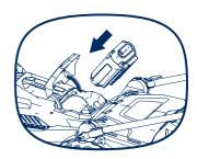
ii. Insert the Safety-Key into assembly hole until you hear a click, then close the battery pack tank cover.
