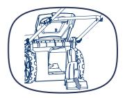
iii.Lift up the rear flap before assembling the grass bag. Hang the collection bag on the mower.
