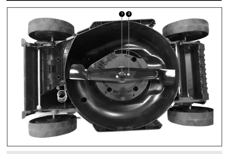
Turn the machine carefully onto its right side and inspect the blade. If blunt or damaged, replace it.
