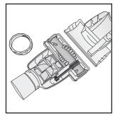
tool transparent cover for cleaning, twist the locking ring to the unlock position and remove it.
