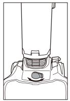
Turn height adjustment knob to adjust from Low to high pile carpet or turn vacuum cleaner on. hard floor setting as appropriate.
