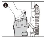
Press release button and lift off dust container.
