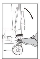
Step on cleaner release Press release button button to lower handle and lift off dust into position for vacuuming floors.
