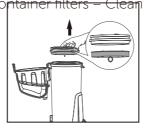
Lift out foam filter and shake off dust Rinse foam filter and dry thoroughly.
