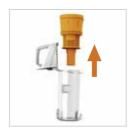
Lift and remove the separator out of the dirt container. Using a soft brush remove any dirt and debris from the separator.
