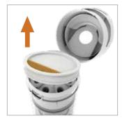
Pull the pre-motor filter tab and remove the filter from the separator.
