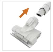
Slide the mini motorised pet tool onto the end of the hose until it clicks into place.
