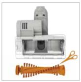
To remove any threads or hair, slide the blade of a pair of scissors into the groove on the brushbar and cut along the groove. Clear any dirt/debris inside the housing of the floorhead.
