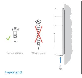
**Note:** For your safety, use only the short security screws under the faceplate. Using any other type of screw could damage the battery and create a potential fire hazard. If you feel that you may have used the wrong screw to install your doorbell, please contact Ring Customer Support.
