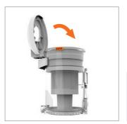
Refit the separator making sure that the tab on the separator fits into the groove on the dirt container.
