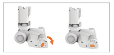
Refit the brushbar into the powered floorhead. Align the arrow on the brushbar cover so it points north, firmly push and twist clockwise to lock.
