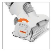
Using a coin, turn the brushbar lock anticlockwise to release the brushbar.
