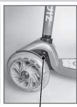
Press the red plastic button for disassembly
