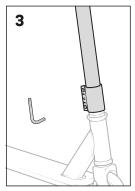
Repeat the process until all screws are securely tightened.
