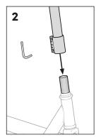
Insert the T-bar onto the fork stem. Tighten the screws with the Allen key from top to bottom.
