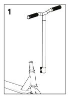
Place the triple clamp over the vertical tube of the T-bar.
