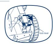
d. Push the scarifying blade cylinder out of the seat.
