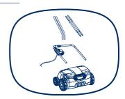
B. Align the lower handle bars with frame (Lower hand bar hole). Keep the direction of both lower handle bar in line with the wheels will assist in aligning the corresponding holes in the frame.
