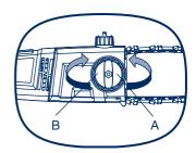
2 Fit the chain around the bar ensuring that the direction of the chain is as depicted in the picture on the bar. Fit the chain on the sprocket.
