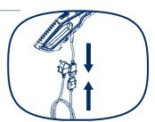
Push a loop of extension cable through the space in the handle and fix the extension cord on cord retainer.
