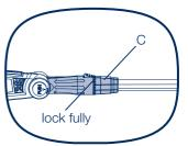
When removing, Push the locker button(D), then turn locker (C) anticlockwise to unlock, then pull the handle out
